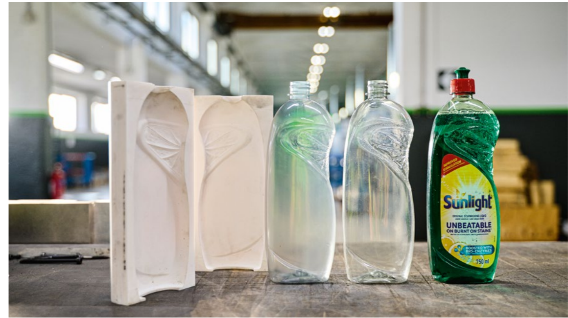
At left: A two-part, 3D-printed mold and a bottle it was used to produce, standing next to a steel mold and a labeled prototype for consumer tests Below: SLA 3D Printing makes it possible to produce molds in just two days
